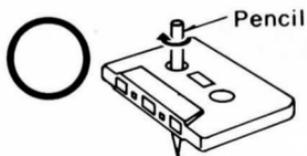
Tape looseness can be corrected by turning a pencil in the direction of the arrow.
